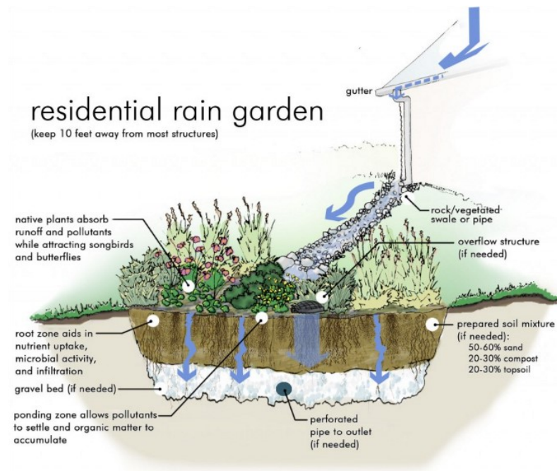
Cross-section of a typical rain garden installation, designed to prevent pollutant runoff and more thoroughly distribute rainwater recharge. Source: Michigan United Conservation Clubs
