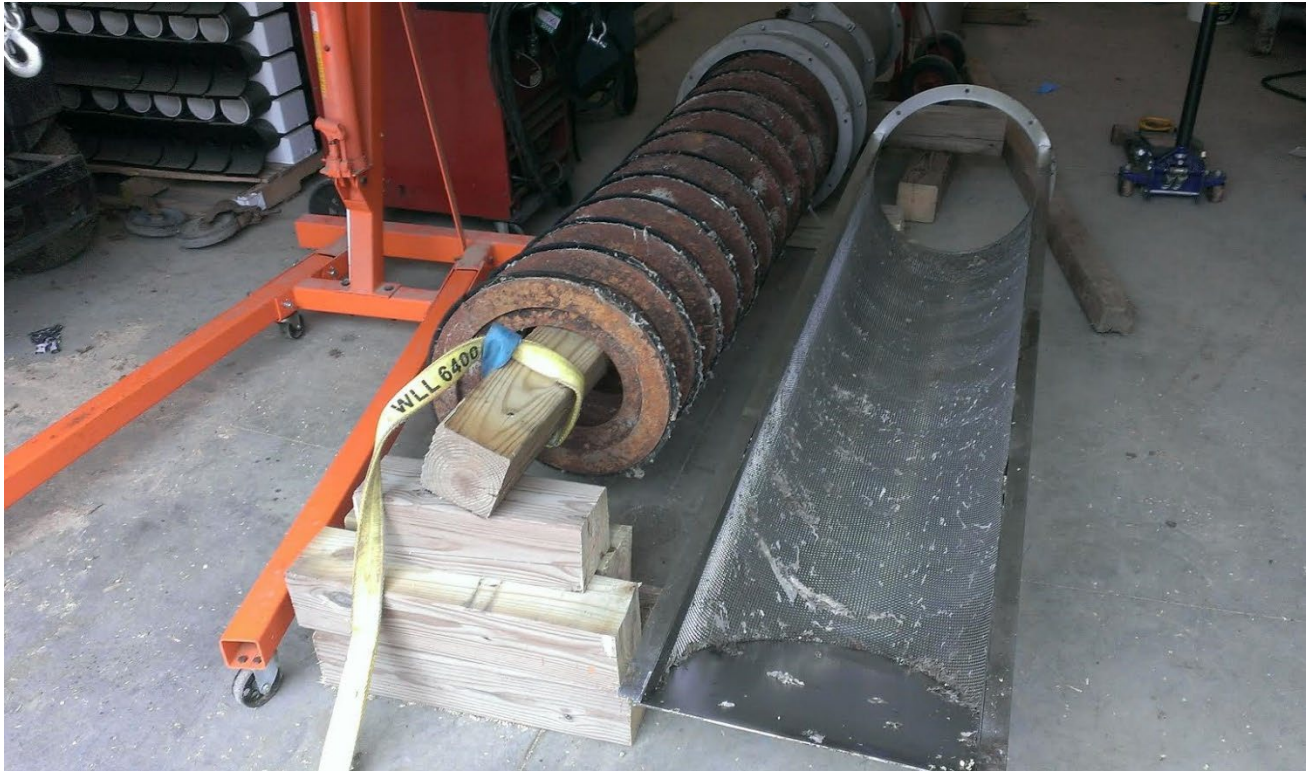
Septage screen and auger screw (with brush)
