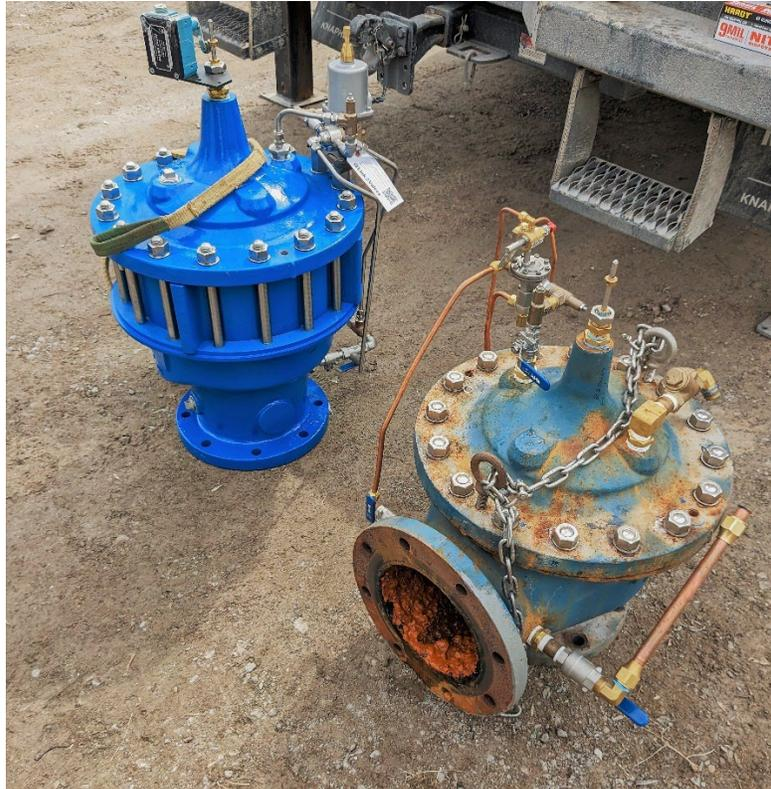
*New PRV (left) and old PRV (right)*
