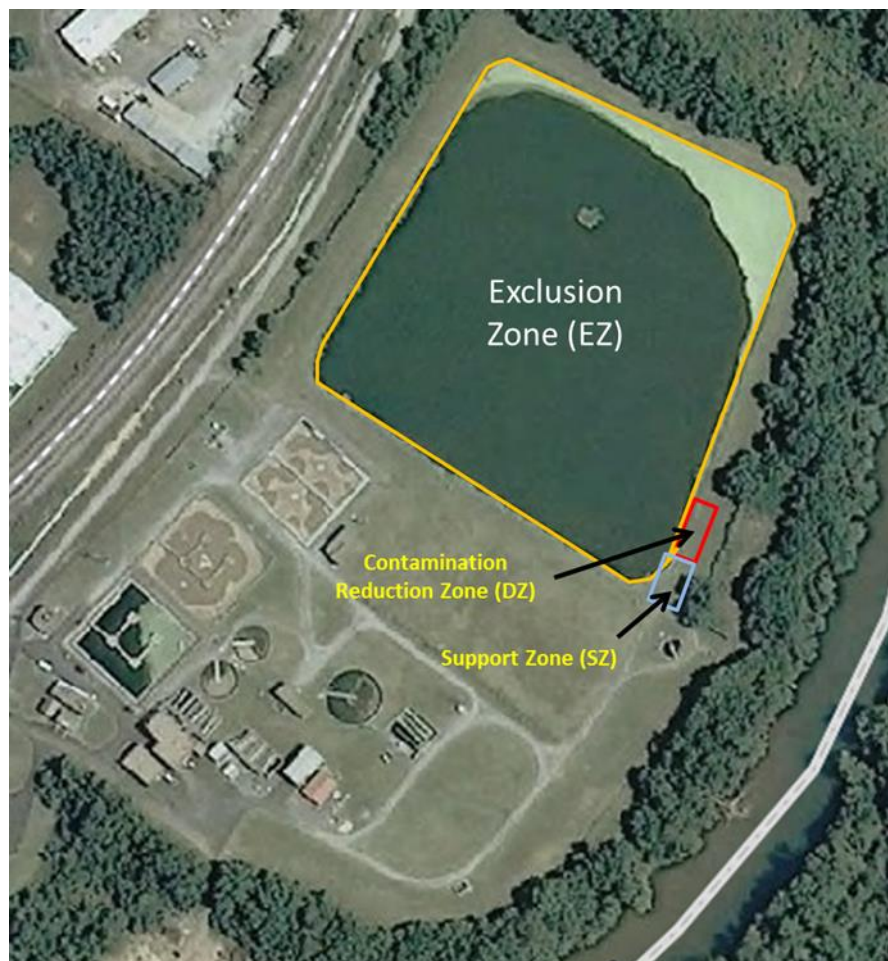
Figure 1 – Site zones are intended to control the potential spread of contamination and to assure that only authorized individuals are permitted into potentially hazardous areas. A three-zone approach will be utilized. It shall include an Exclusion Zone (EZ), Contamination Reduction Zone (CRZ), and a Support Zone (SZ).
