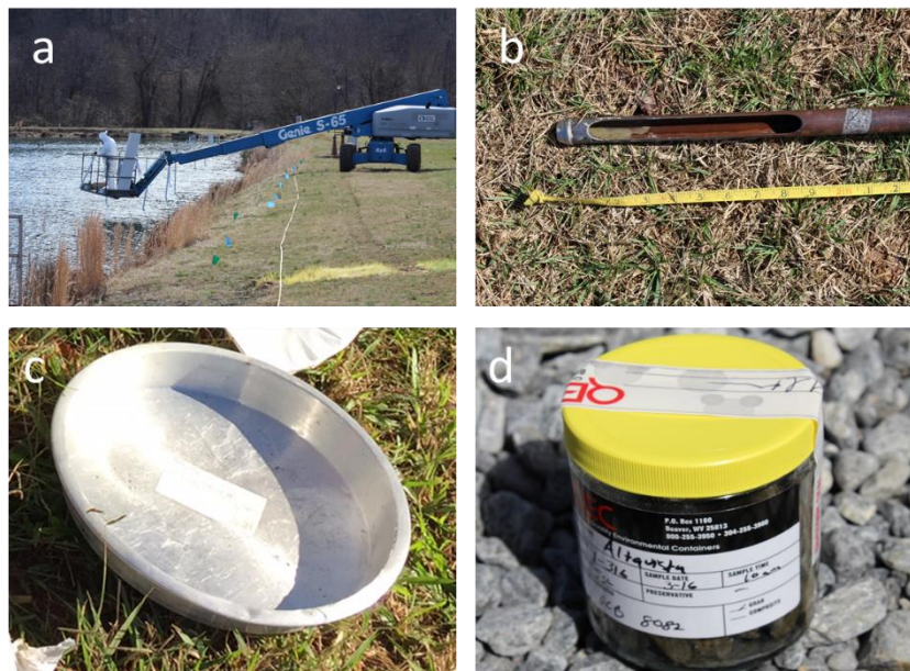
Figure 1. (a) Example of taking samples 10 and 20 feet from the shore on 3/16/15. (b) Sampler used for the pond re-characterization in 2015. (c) 14 inch metal pan used to homogenize each sample. (d) Sample jar with custody seal applied.
