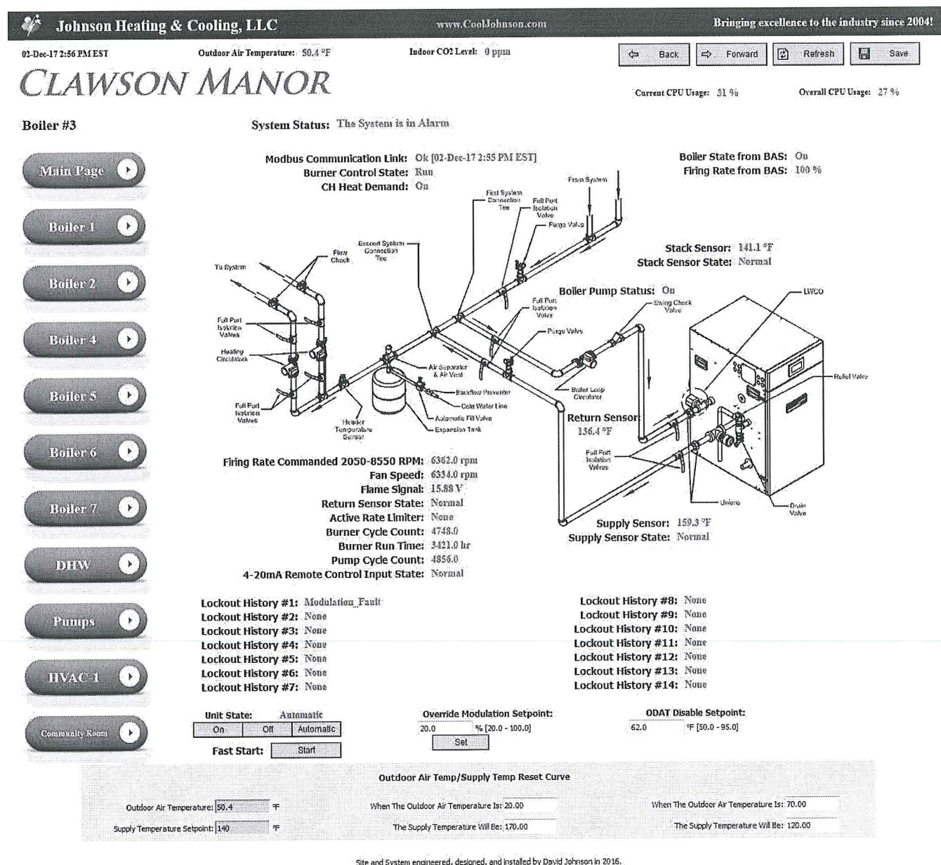
Figure 1- Shows Modbus values from Sage 2 controller, to be displayed on automation system's GUI.
