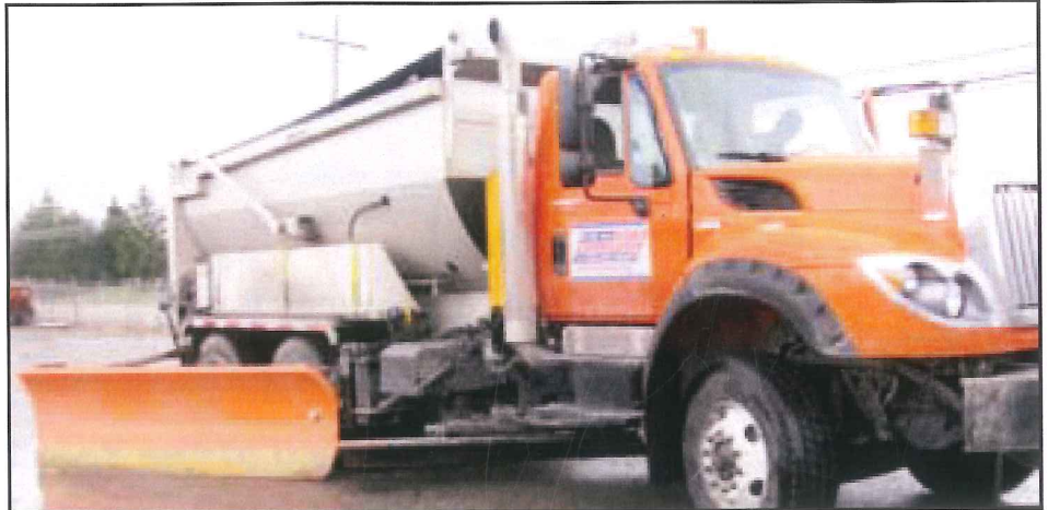
An RCOC plow truck equipped with a wing plow.
