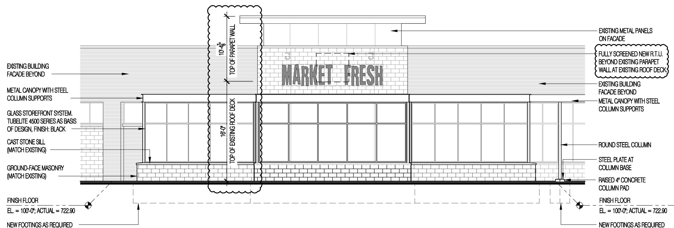
H8 A200 Proposed South-East Elevation (Entry) SCALE: 1/8" = 1'-0"
