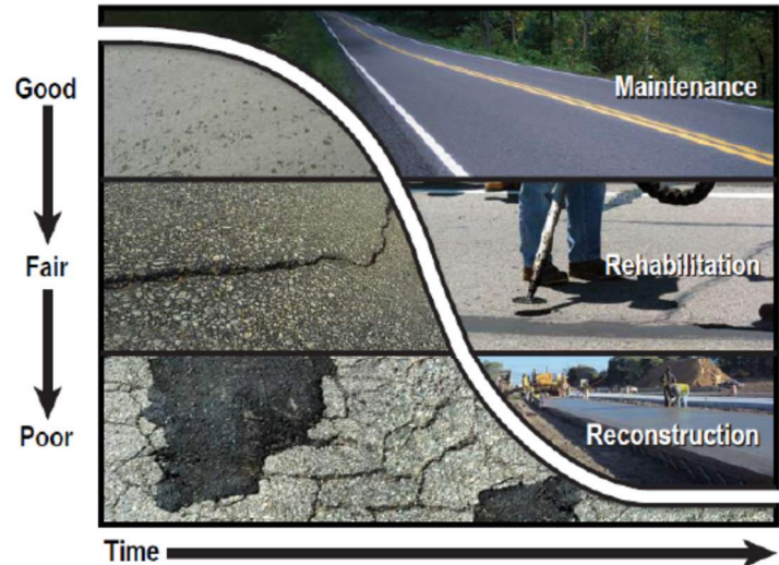
Figure 2 Road Deterioration Curve
