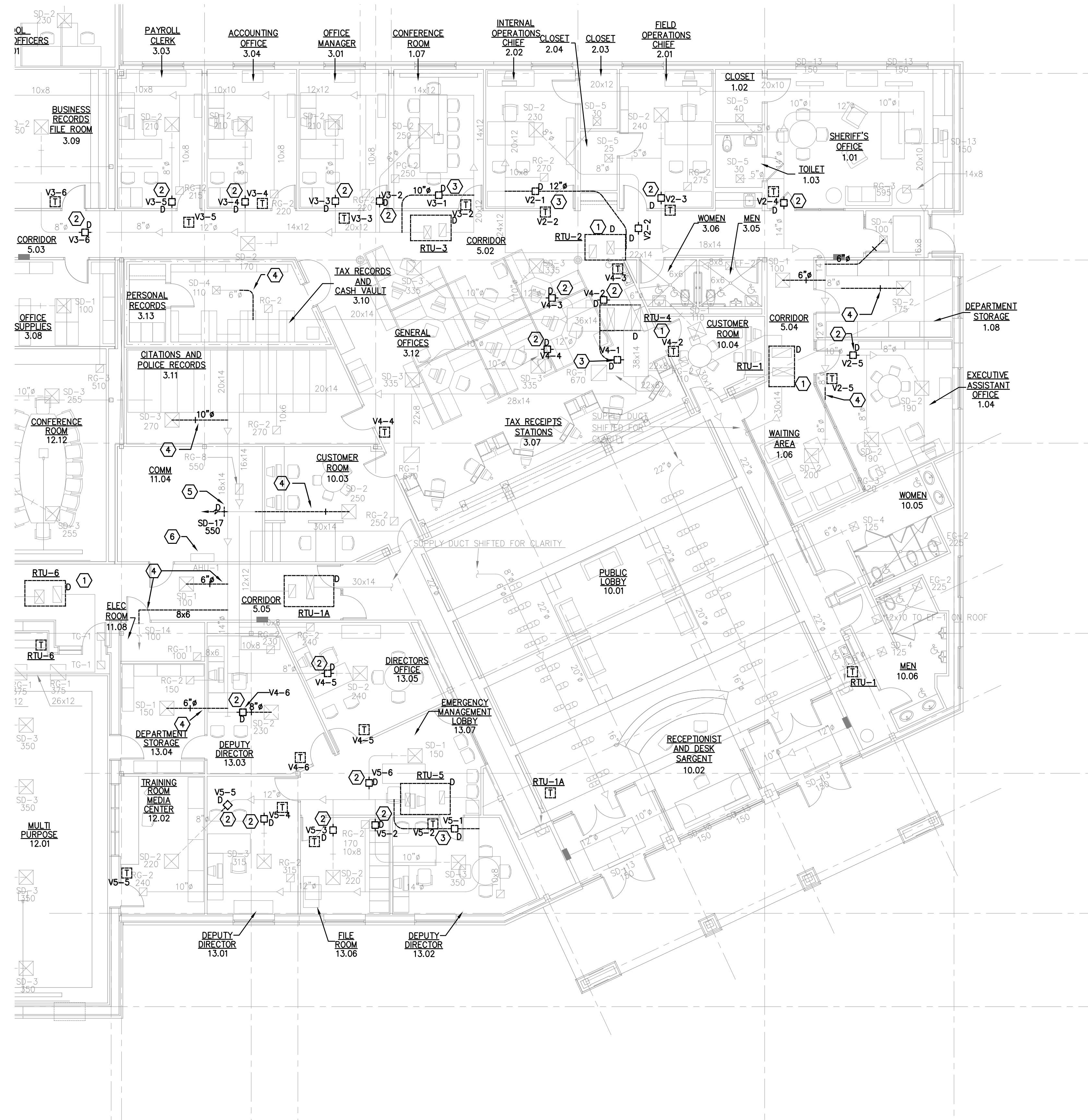
AREA 1 - HVAC DEMOLITION PLAN SCALE: 1/8" = 1'-0"
