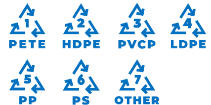
Figure 2. Plastic resin identification codes.
