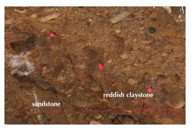
**Photo 8:** Close-up view of the irregular, erosional contact between the reddish silty claystone assigned to the possible Saugus Formation and the overlying Older Alluvial deposits, at about Station 10, near the base of Trench 1a. Note the intensely weathered clasts in the Older Alluvium. Pink flags denote contact. White flag marks sediment sample location used to describe the claystone unit.
