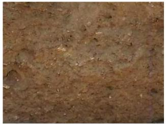
Mudflow deposits in the near-surface were observed from about Station 10 southward to the southern end of Trench 1a, and along the full width of Trench 1b. The sediments consist of dark brown to dark reddish brown (7.5YR hues) gravelly to cobbly sandy loam to sandy clay loam (Photo 12), with subangular to rounded cobbles weathered to Stages 2 to 3.
