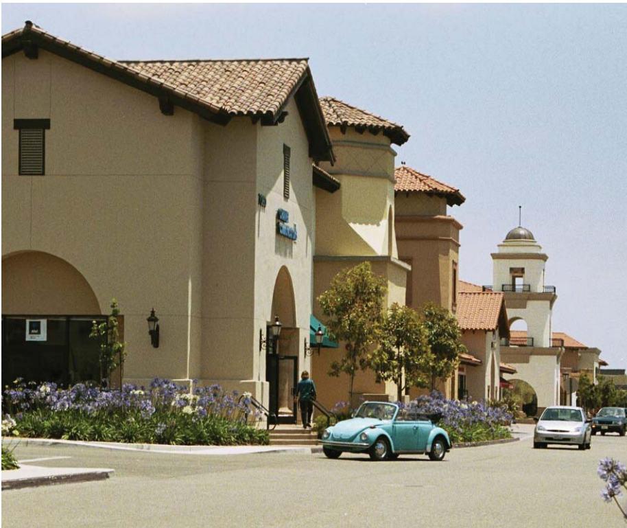
The massing of this building has been broken up by giving the appearance of several buildings joined together
