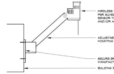
WIRELESS RAIN SENSOR (MODEL PER SCHEDULE) - TOP OF SENSOR TO BE ABOVE GUTTER AND/OR ANY OBSTRUCTIONS
