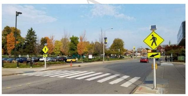
Figure 16: Rectangular Rapid Flashing Beacon (RRFB)
