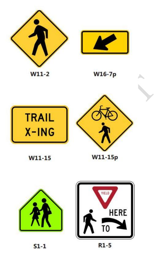
Figure 12: Signage Options (Source: Manual of Uniform Traffic Control Devices (MUTCD))
