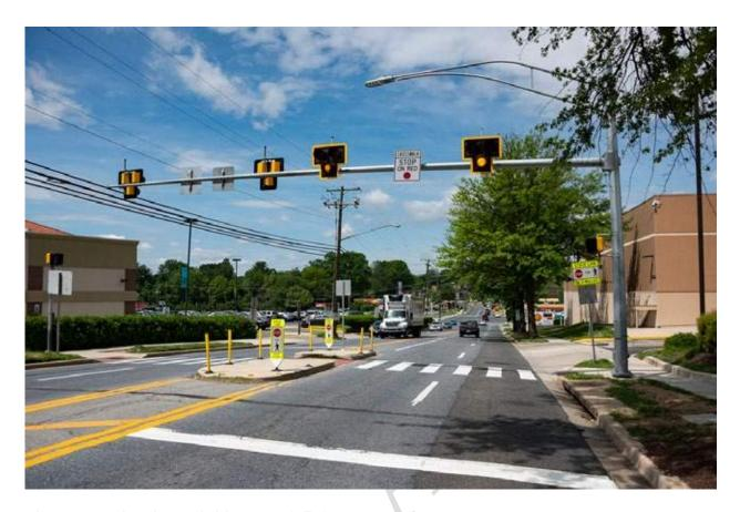
Figure 17: Pedestrian Hybrid Beacon (PHB)
