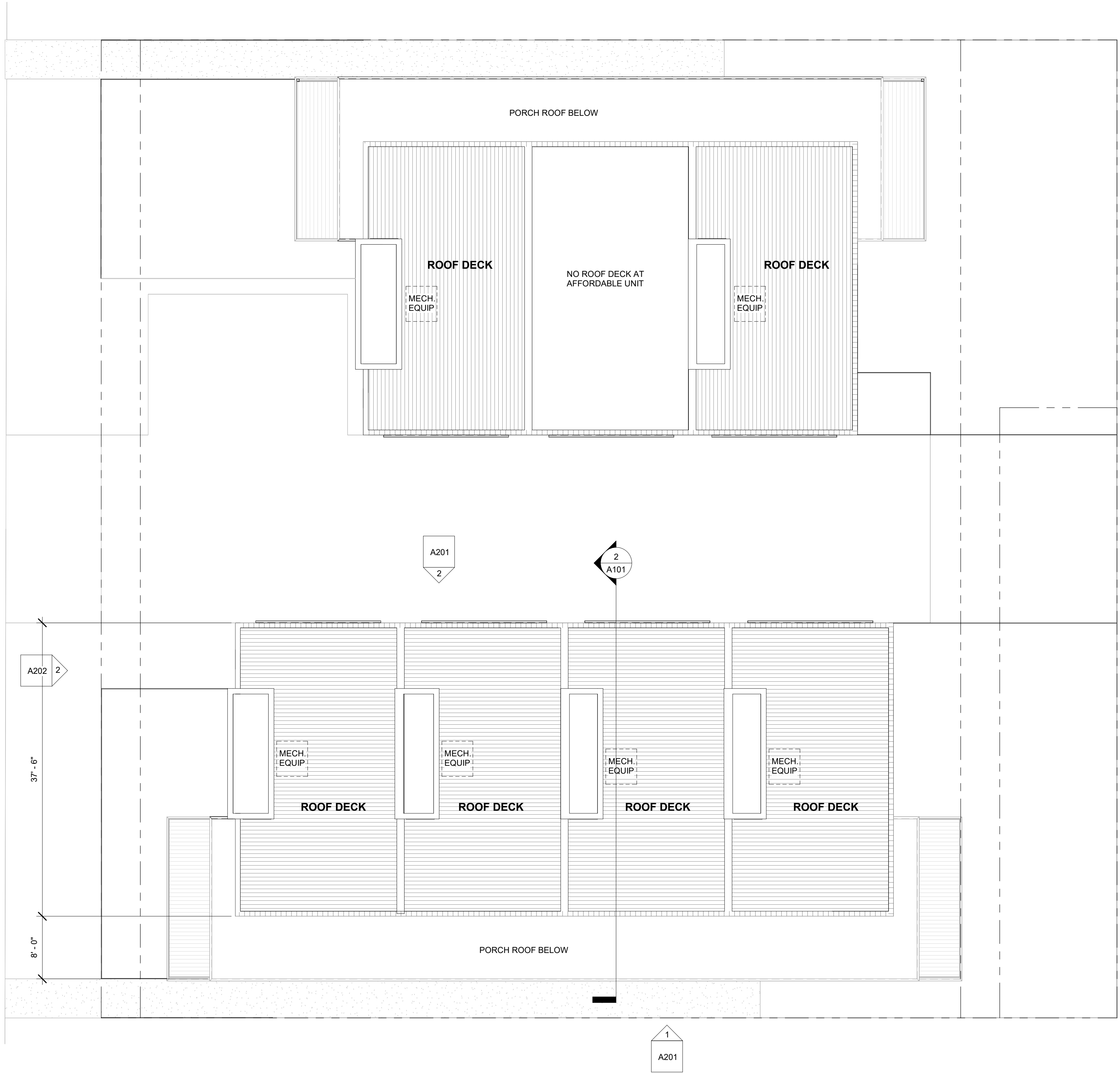
① ROOF DECK PLAN 1/8" = 1'-0"
