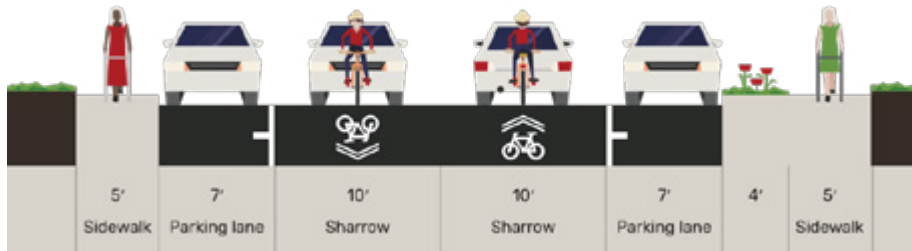
Figure 5: Proposed Cross Section for Colorado Avenue
