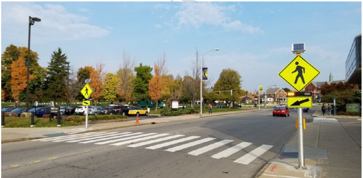
Figure 16: Rectangular Rapid Flashing Beacon (RRFB)
