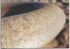
The sand colored variant is made of rotomolded stone mixed PE material with non skid surface texture. Minor differences in the stone mix visuality of the material are to be expected.
