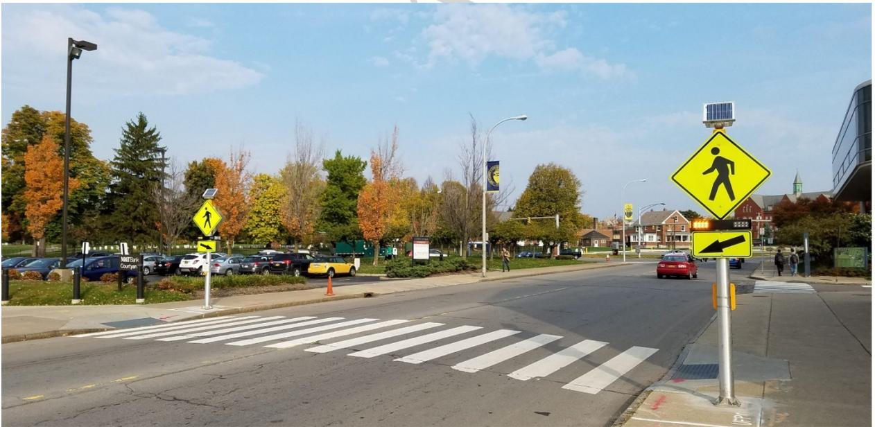
Figure 16: Rectangular Rapid Flashing Beacon (RRFB)
