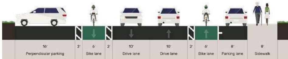
Figure 11: Proposed Cross Section for 2 nd Street (Angled Parking Present)
