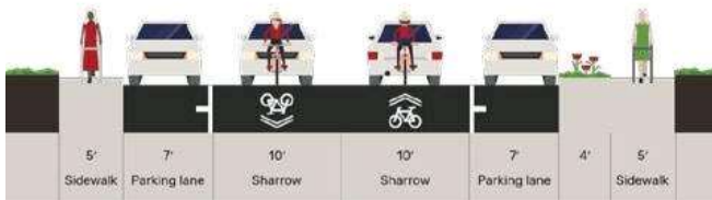
Figure 5: Proposed Cross Section for Colorado Avenue
