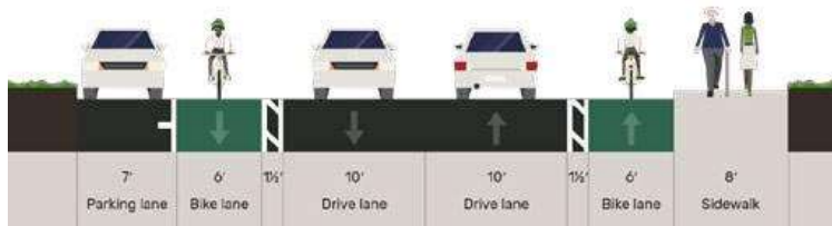
Figure 11: Proposed Cross Section for 2 nd Street (Angled Parking Present)
