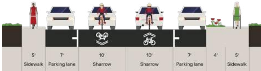
Figure 5: Proposed Cross Section for Colorado Avenue
