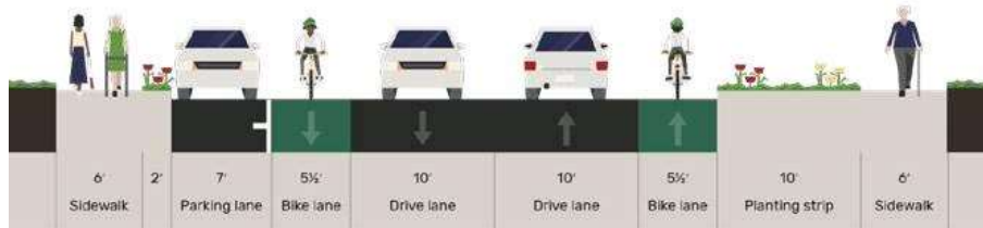
Figure 3: Proposed Cross Section for Hendrick Drive
