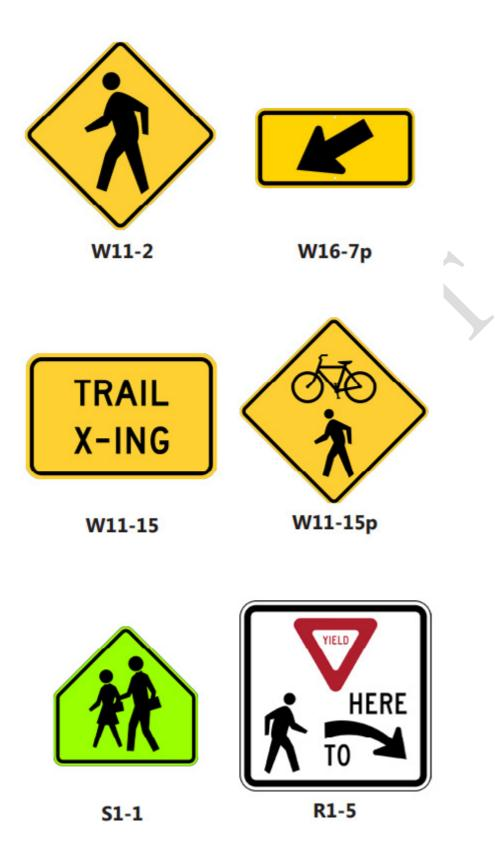
Figure 12: Signage Options (Source: Manual of Uniform Traffic Control Devices (MUTCD))
