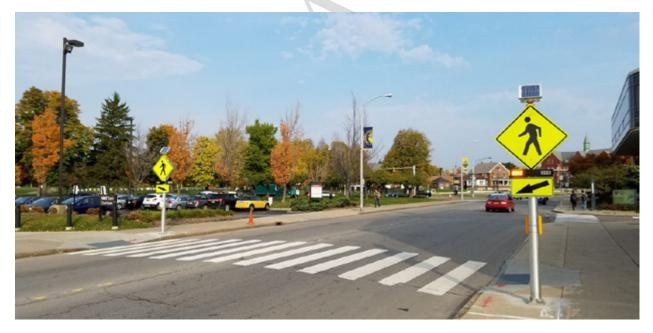
Figure 16: Rectangular Rapid Flashing Beacon (RRFB)
