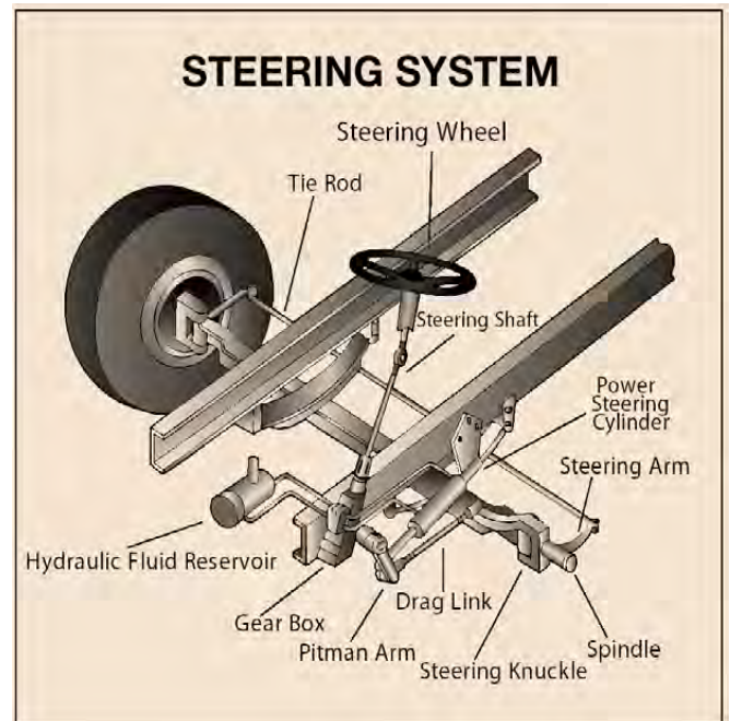
Figure 2.1 illustrates a typical steering system
