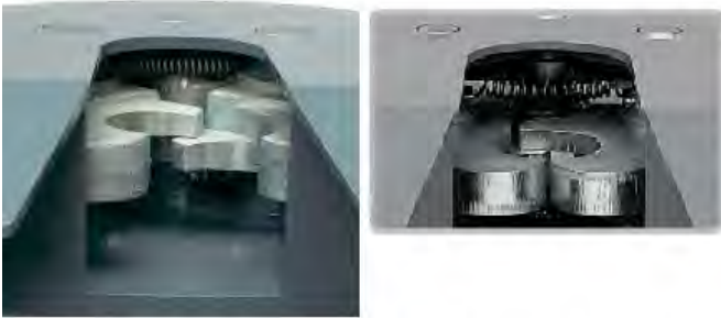
Fifth Wheel Locking Jaws: OPEN CLOSED
