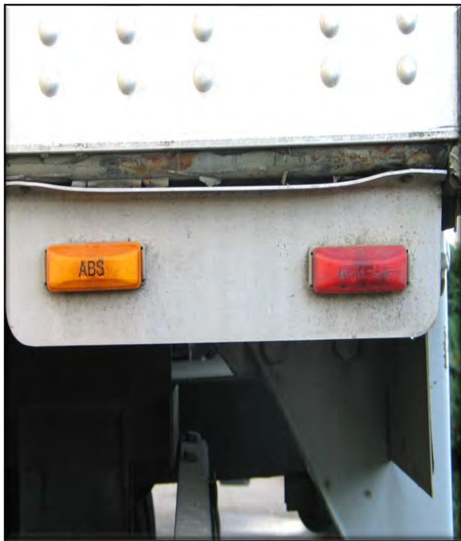
Figure 6.7 – ABS Malfunction warning Light.
