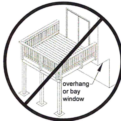
Figure 18. No Attachment to House Overhang with Ledger.
