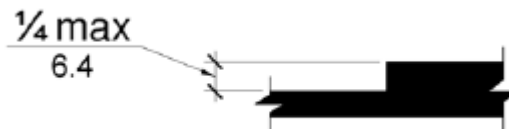
Figure 303.2 Vertical Change in Level
