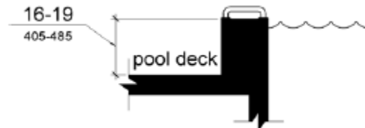
Figure 1009.4.2 Transfer Wall Height
