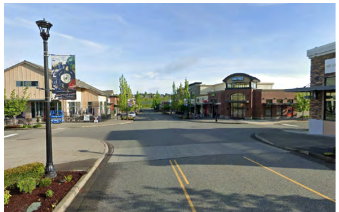
Figure 8-4: Narrow street right-of-way and narrow crossing distances in Snoquamie Ridge, Washington (Source: Google)
