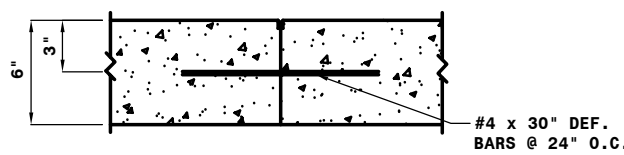
6 TYPE 'C' TIED CONSTRUCTION JOINT DETAIL C7.1 NOT-TO-SCALE
