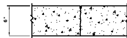
5 TYPE 'H' CONSTRUCTION JOINT DETAIL C7.1 NOT-TO-SCALE
