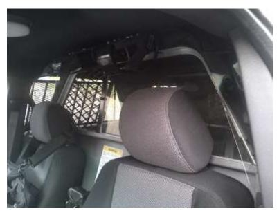
No gaps exceeding 1" from the top, 3" on the side and 4" on the bottom will be accepted. In addition, partition shall not interfere with side curtain air bags and seat belt safety systems.
