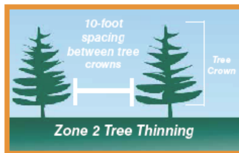
Figure 17: In Zone 2, make sure there is at least a 10-foot spacing between tree crowns. Credit: CSFS
