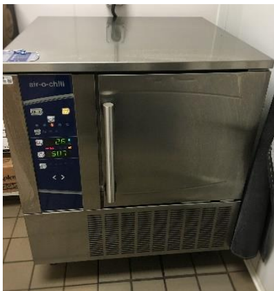
Exterior of Blast Chiller
