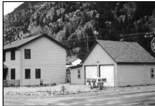
Construct an accessory structure that is subordinate in scale and character with the primary structure. This one is too big compared with the primary structure.
