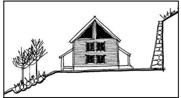
Minimize cut-and-fill that would alter the perceived natural topography of the site. This excessive cut and retaining wall is inappropriate.
