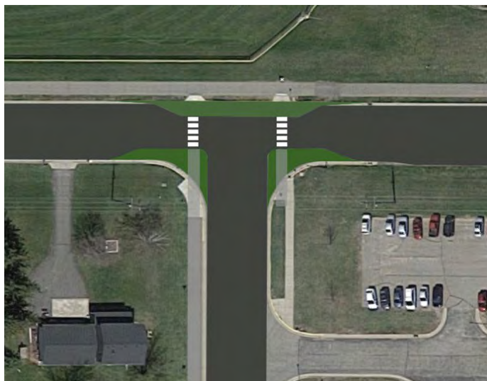
Recommendation B. 16th St NE and 5th Ave NE. Current (left) and recommended (right). Installing curb extensions and additional high visibility crosswalk will improve safety and comfort at an intersection with high pedestrian volumes.
