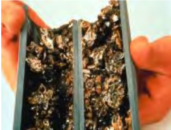
Figure 4-25 Mussels Clogging a Pipe
