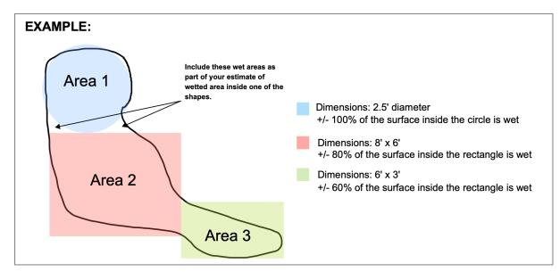
STEP 3: Calculate the area of the footprint by completing the table below for each area in Step 2. Measure actual depth of standing sewage whenever possible. When depth varies, measure several representative sample points and determine the average. If the depth is not measurable because it is only a wet stain, use the following estimated depths: Depth of a wet stain on concrete surface: 0.0026' (1/32")
