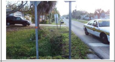
At the intersection of Pinellas Trail and Rosery Rd, looking north. The existing drainage along the north side of the street will need to be addressed during road reconstruction to allow for proper bicycle and pedestrian access to the trail.
