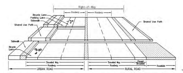
Figure 1: Roadway Right-of-Way
