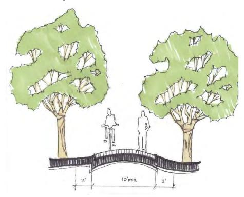
Figure 24: Shared Use Path/Trail Cross Section
