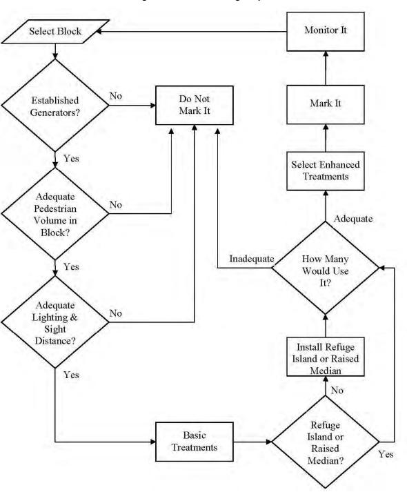
Figure 8: Midblock crossing component flowchart
