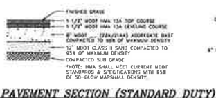
HMA PAVEMENT SECTION (STANDARD DUTY) NO SCALE
