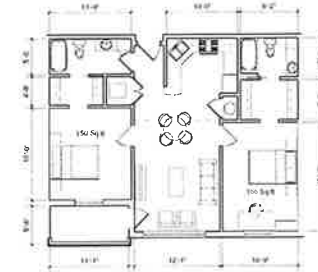
5. Typical 2-Bed Apartment Plan SCALE: 1/8" = 1'-0" NET AREA: 906 SQ FT SECTION 8 04 - DISTRICT REGULATIONS MINIMUM FLOOR AREA: 500 SQ FT PLUS 150 SQ FT PER BEDROOM OFA PER UNIT
