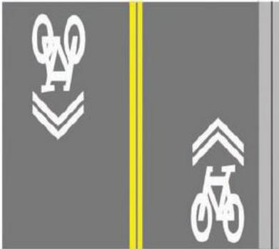
**Photo 9.6: Example of shared lane pavement markings**
