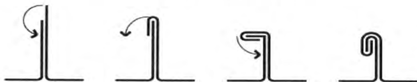
FORMATION OF STANDING SEAM IN TRADITIONAL METAL ROOFING (DOUBLE LOCK SEAM)
