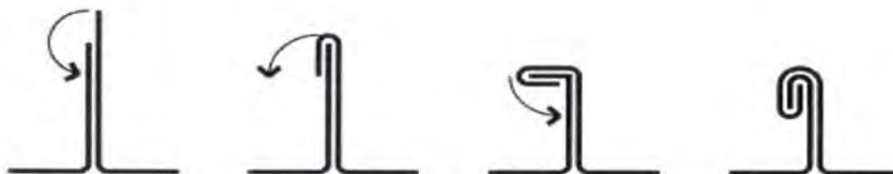
FORMATION OF STANDING SEAM IN TRADITIONAL METAL ROOFING (DOUBLE LOCK SEAM)
