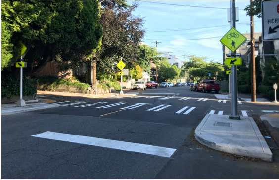
Rectangular rapid flashing beacons (RRFB) alert drivers at unsignalized intersections of people biking or walking.
