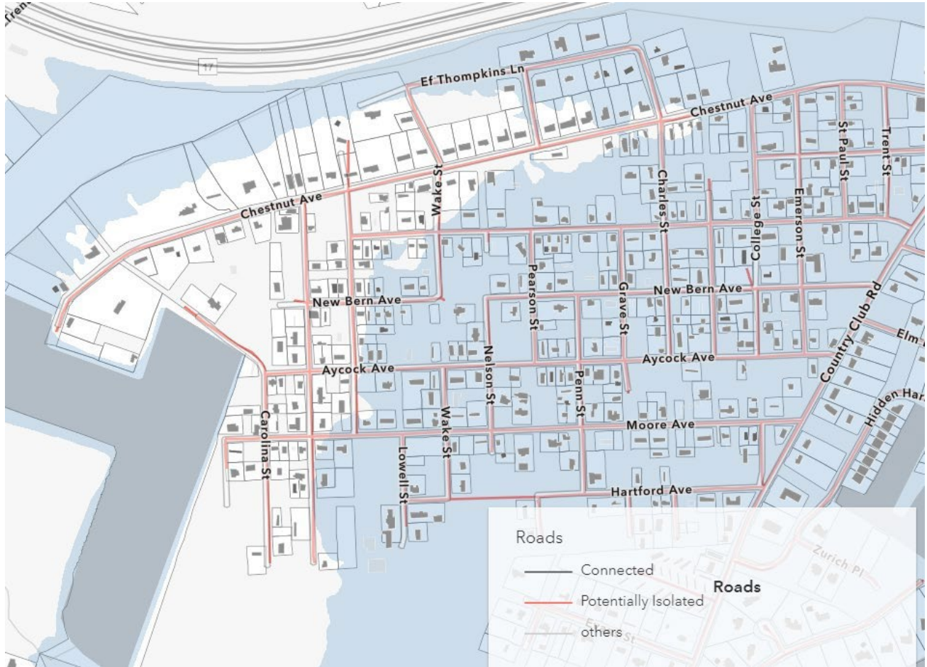
Figure 7.15. Illustration of roads and properties potentially inaccessible to 100-year floodplain inundation (top) and a map showing the number of all properties potentially inaccessible within for the study (bottom)
