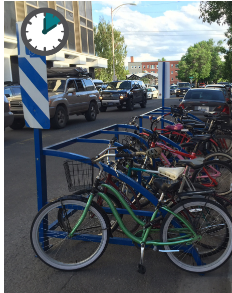
Tier 2A: Bicycle Corral: Bicycle corrals provide high-capacity parking outside of the pedestrian zone, helping to minimize sidewalk clutter. This rack type should be installed at locations with high demand, such as at shopping plazas or near restaurants. Many corrals are designed to fit conveniently within one conventional vehicle parking space.
