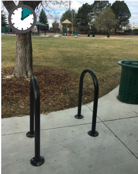
Tier 1: Short-Term Bicycle Parking: Short-term bicycle parking is to be placed on sidewalks in front of higher turn-over establishments, or near the entrance to buildings on private property.
