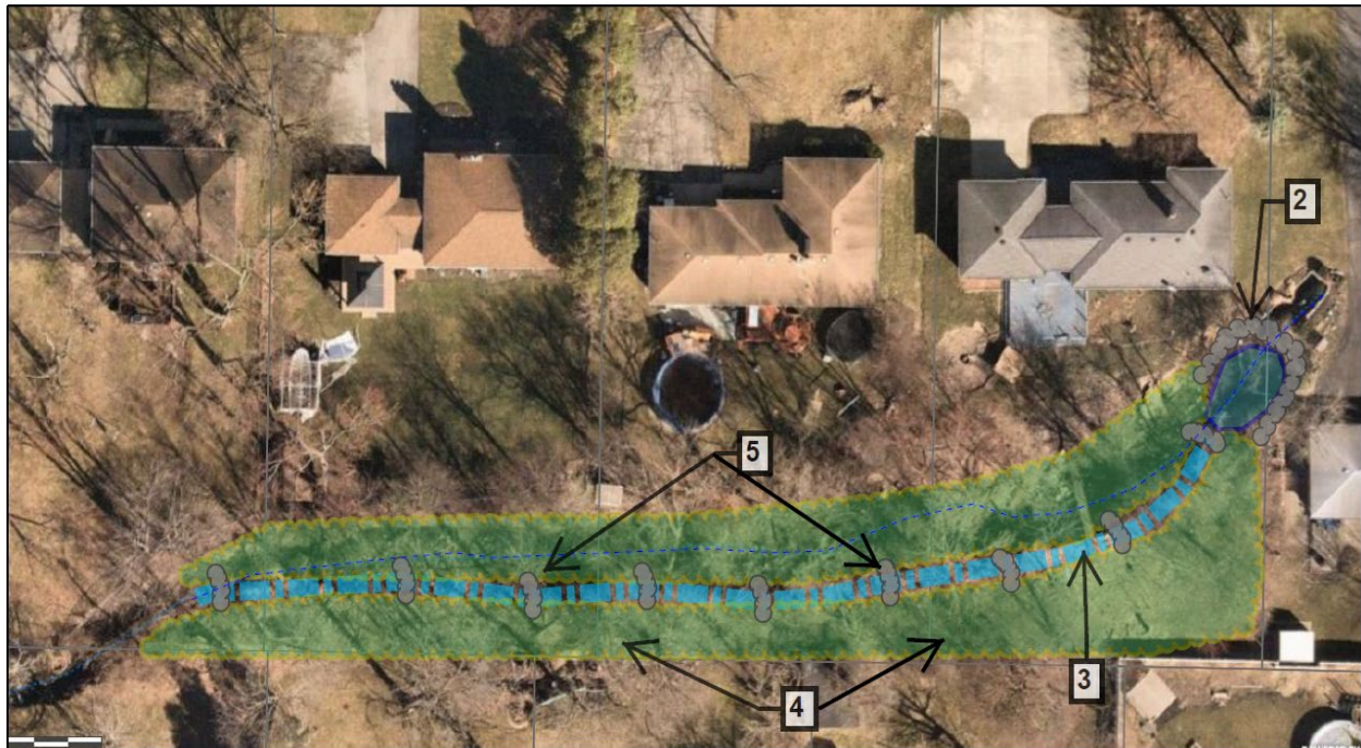
Figure 2 Potential stabilization improvements along the stream channel.
