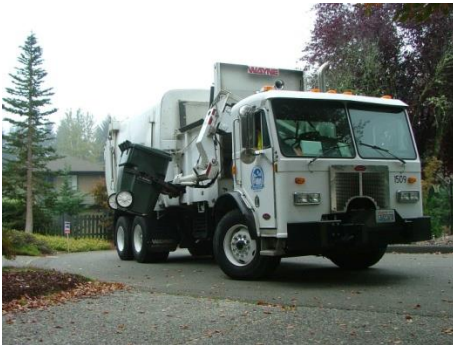
Figure 3: Automated side-load Residential collection and multi-family recycling
