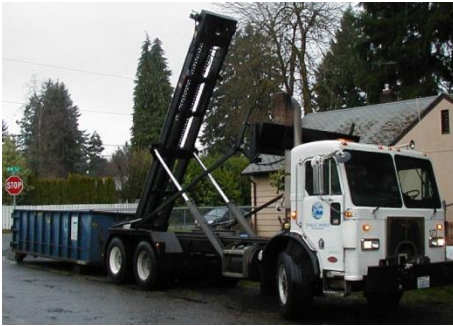
Figure 1: Tilt frame drop box “roll-off” truck
