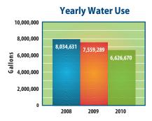
The hospital completed an extensive water-efficiency retrofit, replacing 131 toilets, 105 showerheads, and 233 faucet aerators with high-efficiency fixtures. This major water conservation project saves 2,555 gallons of water per day, helping to protect drinking water resources and reducing wastewater
