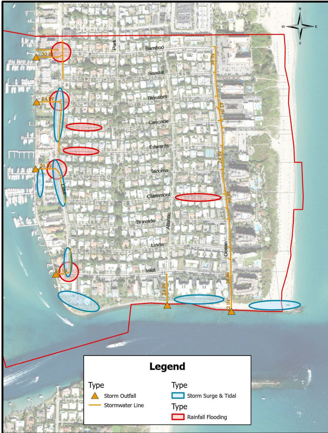
Figure 6: Tidal and Stormwater Flooding Areas of Concern
