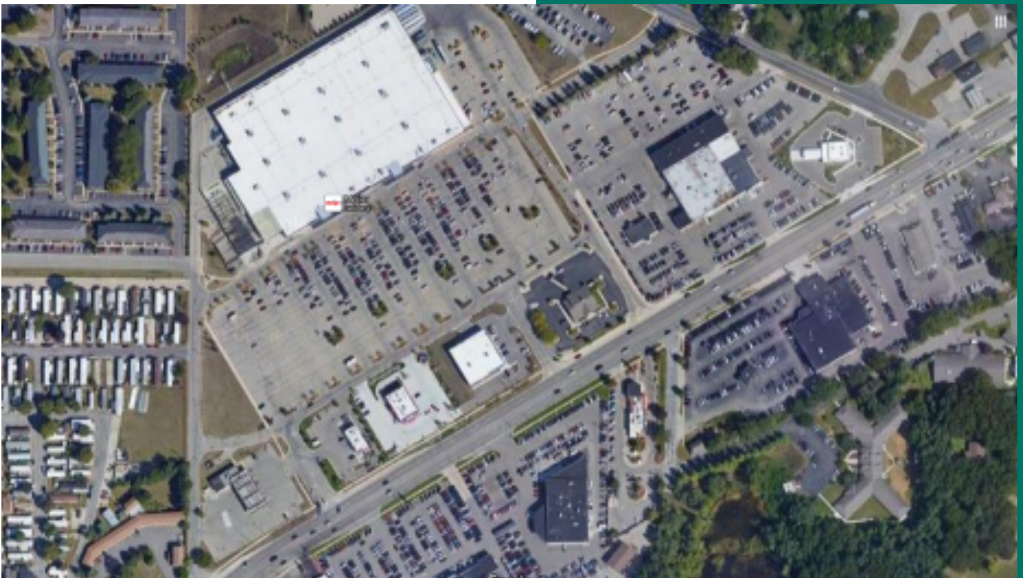
This image of Meijer, its outlots, car dealerships, and roads illustrate the many acres of asphalt and rooftops that are present along Plainfield Avenue. The area is largely devoid of trees and stormwater is collected through pipes then discharged into the Grand River.
