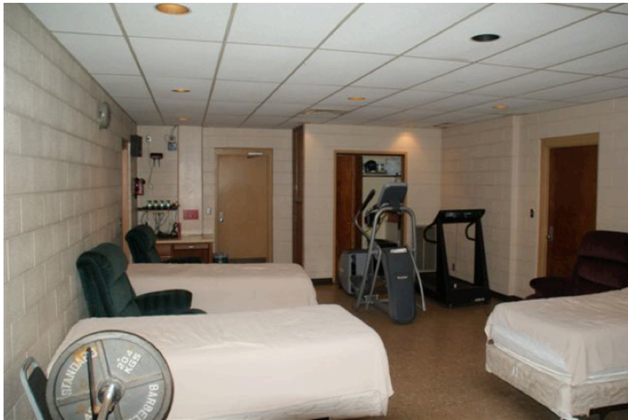
The door at the far end leads directly to the apparatus floor. There should be a transitional corridor to the apparatus floor. The door to the right is an unmarked exit door leading to a vestibule at the back entrance.
