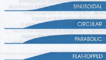
Figure 1. Graphic. There are several options for raised crosswalk profiles. The sinusoidal profile (top example) is easiest for snowplows to maneuver due to its curving slope that transitions gently from the road surface to the top of the raised crosswalk.
